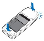
6 Position the back cover over the locking catches on both sides of the phone and slide toward the top of the phone.
